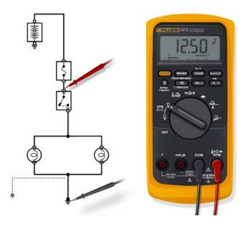
An example is when a short-to-ground occurs within a circuit after the load. The circuit could remain unaffected by that type of failure.
