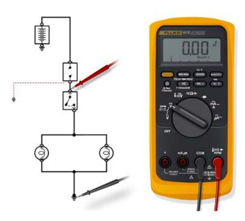
**CAUTION:** Never replace a fuse or circuit breaker with one that has a higher amperage rating.
